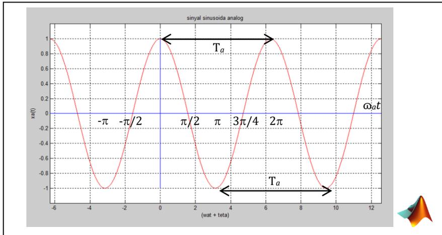
**Gambar 2.1 Fungsi Sinusoida  $x_a(t) = A \cos \omega_a t$ ,
