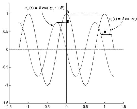
**Gambar 2.3 Sinyal  $x_a(t) = B \cos(\omega_a t + \theta)$
