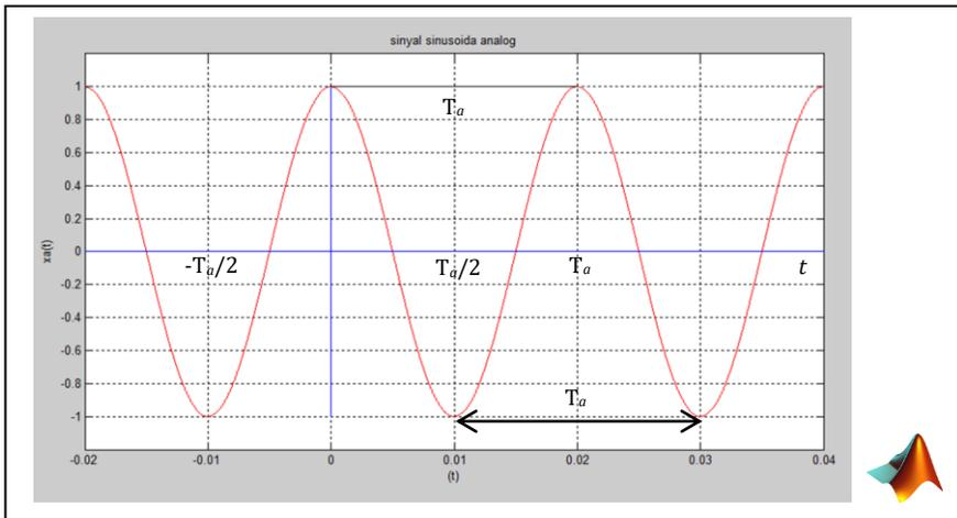
**Gambar 2.2 Fungsi Sinusoida  $x_a(t) = A \cos \omega_a t$
