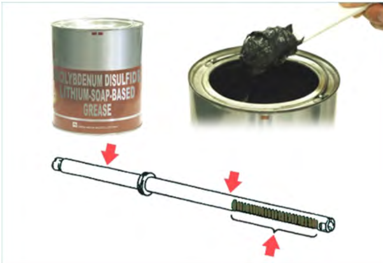
Gambar 5.10. Gemuk berbahan dasar sabun molybdenum disulfide lithium Sumber: team21 toyota
